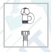
1. Connect the inlet hose by screwing it to a cold water tap using a 3/4 gas threaded connection (see figure).
